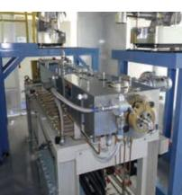
Twin-screw extruder with excellent formance in mixing high-viscosity substances and heat removal
